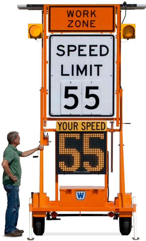
Large Folding-Frame Speed Trailer with optional flashing beacons
