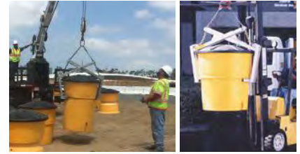
Easy lift with Lifting Ring
