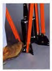
Place right foot on both release levers located between the legs and step down. Both legs will fall to the ground.
