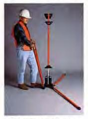
Walk to the other side of the Little Buster stand, place your left foot on both release levers and step down. The remaining two legs will fall to the ground.
