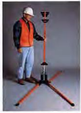
Once all four legs are firmly on the ground, pull-up on the mast to lock legs in place.
